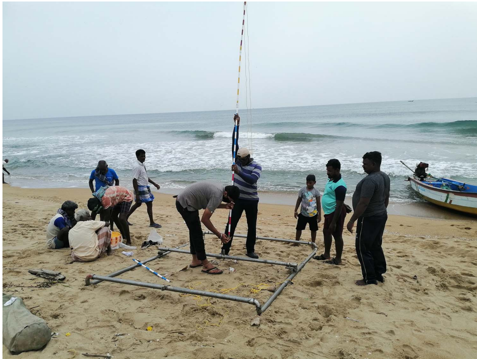
Figure 5. Assembling of the wave sled at the shore is shown, as taken during the field observations.
